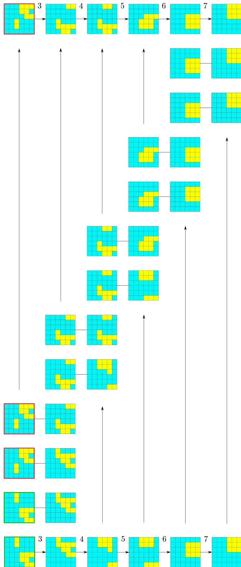
FIGURE 4.7: Conversion of the ordered list of class representatives (obtained from the state enumeration tree) to generate an actual move sequence of states.
