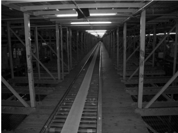
Figure 2: A photograph of an empty picking line showing the conveyor belt in the middle and the bay locations to the left and right of it.
